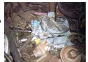
spec or worn metering rods can cause damage to the catalyst. Also, check the choke system to make sure it is operating properly and if the carburetor is an electronic feed back modle, make sure all adjustments are made according to manufacturer specs. Also make sure all feedback sensors and electronic components, such as mixture control solenoids, throttle position sensors and throttle holding solenoids are operating and are within specs.
