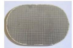
When the engine burns a lean air/fuel mixture, high amounts of oxygen from the exhaust stream flow through the substrate of the catalytic converter. The washcoat on the substrate absorbs this excess O<sub>2</sub> and stores it for use during rich air/fuel mixtures when it is released to help in the oxidation process.
