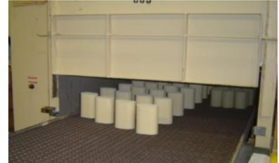
The definition of a catalyst is: a material which increases the rate of a chemical reaction while it is treated during the noble metal and washcoat process, it passes through an oven process which removes excess water and calcines in the substrate. This means it removes all traces of the chemical carriers which are used to deposit the noble metals during the preparation of the catalyst.
