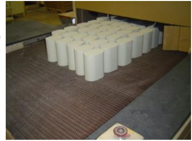
3. NOBLE METALS These are the commonly used elements; platinum, palladium and rhodium, and are deposited onto the washcoated substrate. These metals are what serve to cause the catalytic reaction.
