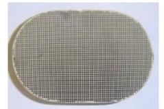
c. **METALLIC FOIL SUBSTRATE** This type of substrate uses wound or stacked metal foil on to which the washcoat and noble metals are deposited. The exhaust gas flows through this substrate. This type has many advantages over ceramic, such as, being able to be made into shapes that cannot be easily done with ceramic.
