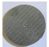
d. **CERAMIC FOAM** This type of substrate is composed of ceramic solution on foam. It is then fired in a kiln to develop the multipore design seen in this photo. This substrate is then treated with washcoat and noble metals. As the exhaust gasses flow through it, the catalytic reaction takes place.
