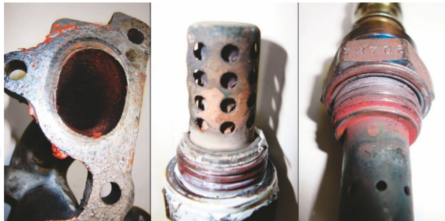
Typical contamination problems (left to right) silicone used on exhaust manifold, O 2 sensor contamination from Teflon Tape, and silicone contaminated O 2 sensor.
